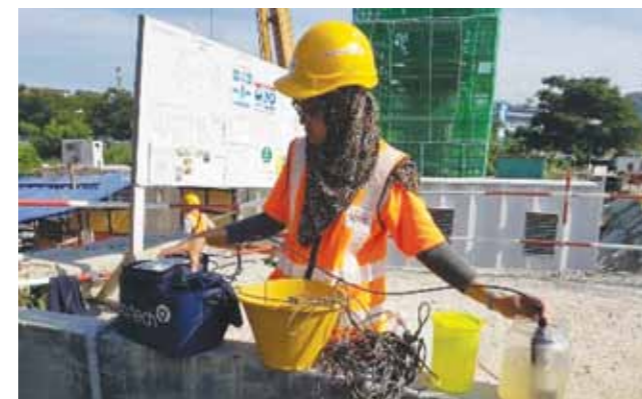
In Situ Total Suspended Solids and Water Turbidity Testing
